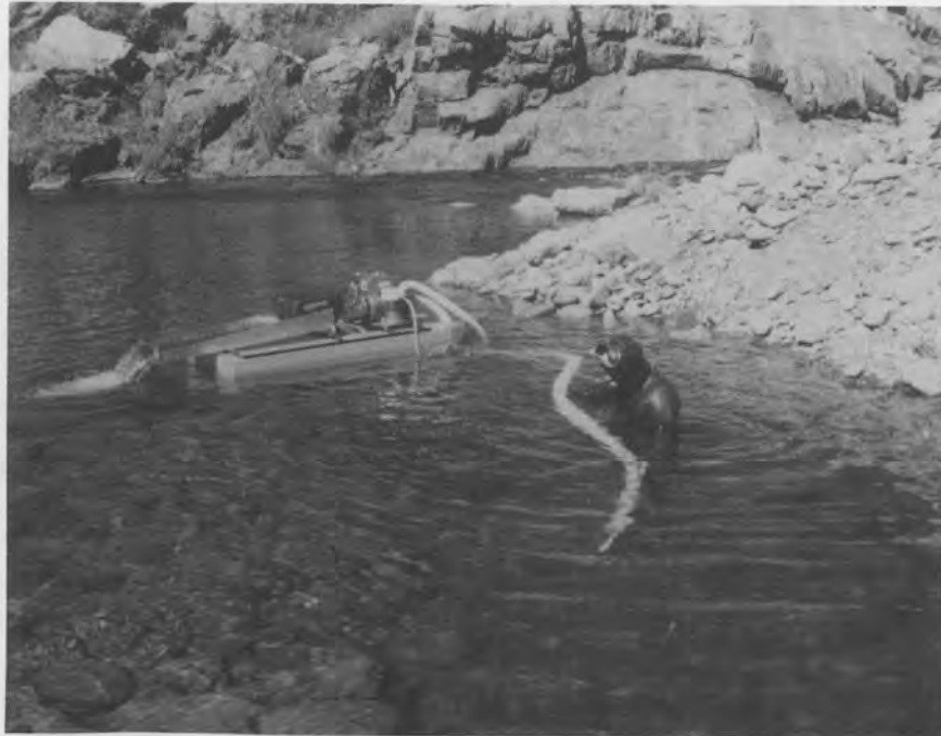
Diver scans bedrock for seams of gold, which are often covered with surface soil.
