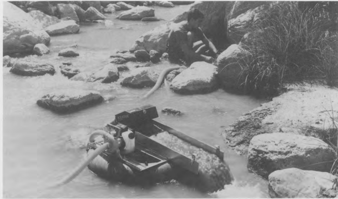
Diver with dredge and sluice at work.
